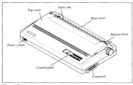
Figure 1-2. The printer's external parts
