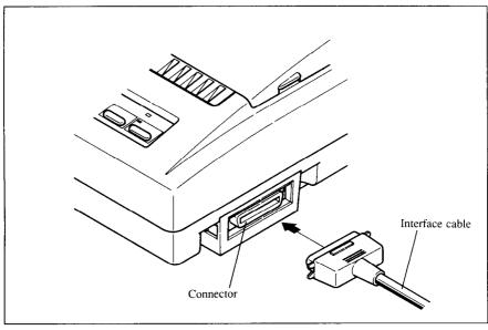
Figure 1-7. Connecting the interface cable
