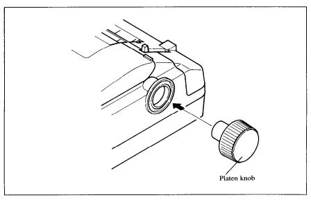
Figure 1-3. Mounting the platen knob
