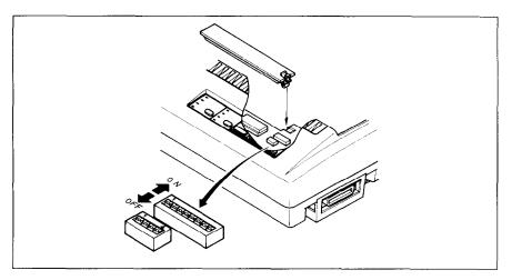
Figure 3-1. DIP switches
