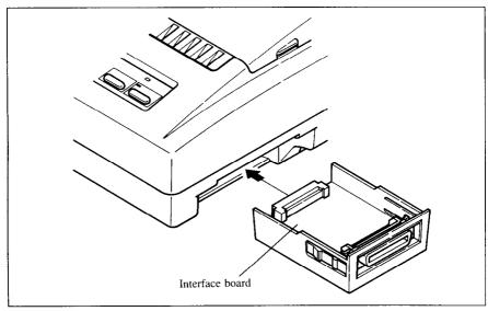
Figure 1-8. Replacing the interface board
