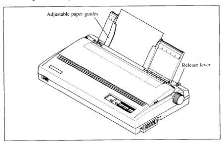
Figure 1-10. Loading a single sheet
