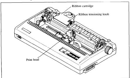
Figure 1-5. Installing the ribbon cartridge
