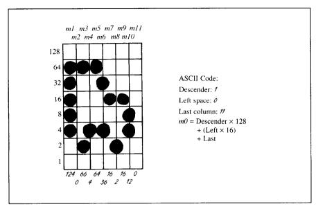
Figure 5-3. Add the values of the dots in each column and write the sum of each column at the bottom
