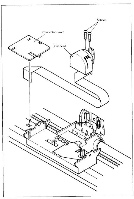
Figure 7-1. Replacing the print head
