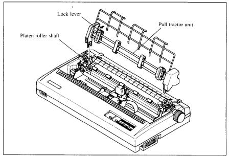
Figure 1-14. Mounting the optional pull tractor unit
