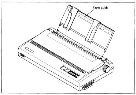
Figure 1-9. Mounting the paper guide for single sheets
