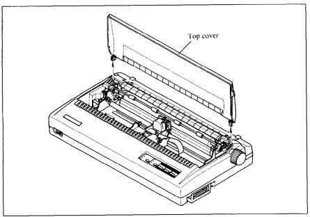
Figure 1-4. Removing the top cover
