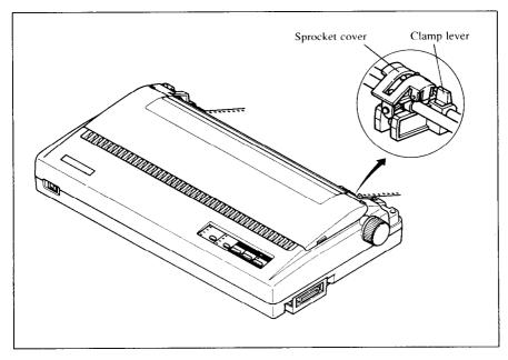
Figure 1-12. Thread the fanfold paper over the sprockets.
