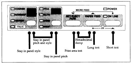
Figure 2-2. Power-up functions of control panel
